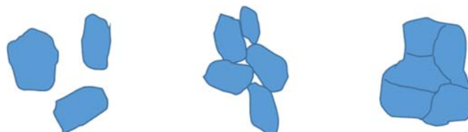
Figure 1: Particles in unbound (left), agglomerated (middle) and aggregated (right) states.
